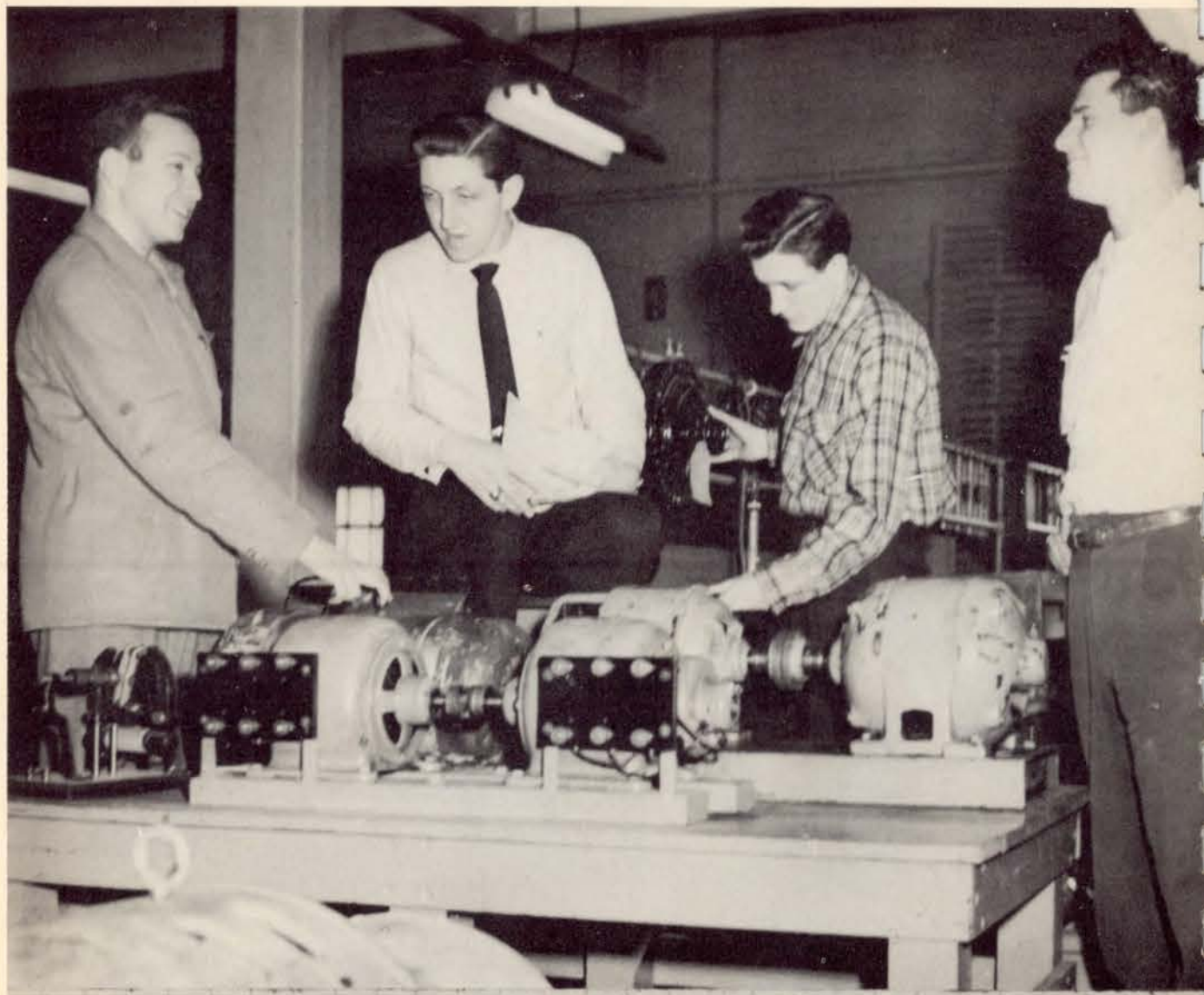
Studying the external characteristics of a D.C. generator. (J. Burch, J. Bodnar, D. Brodowski, P. Scozzari.)
